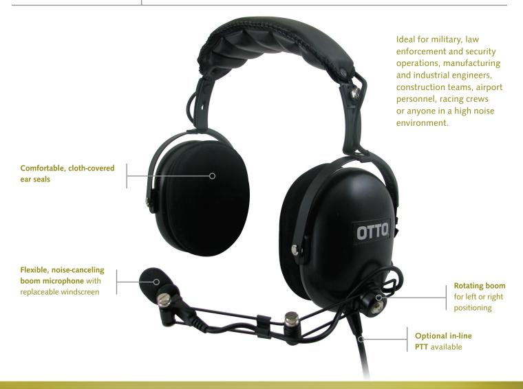
OTTO Over-the-Head heavy duty headsets are Mil-Spec and IS/ATEX certified and deliver comfort, reliability and protection. Microphone position can be adjusted by rotating the boom left or right. The headsets offer a certified noise reduction rating (NRR) of 24dB and provide high clarity audio and additional hearing protection necessary for consistent, clear communication in extreme noise environments.
